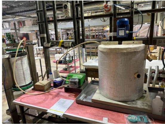
Figure 1: MREC precipitation tank and setup at ANSTO.
